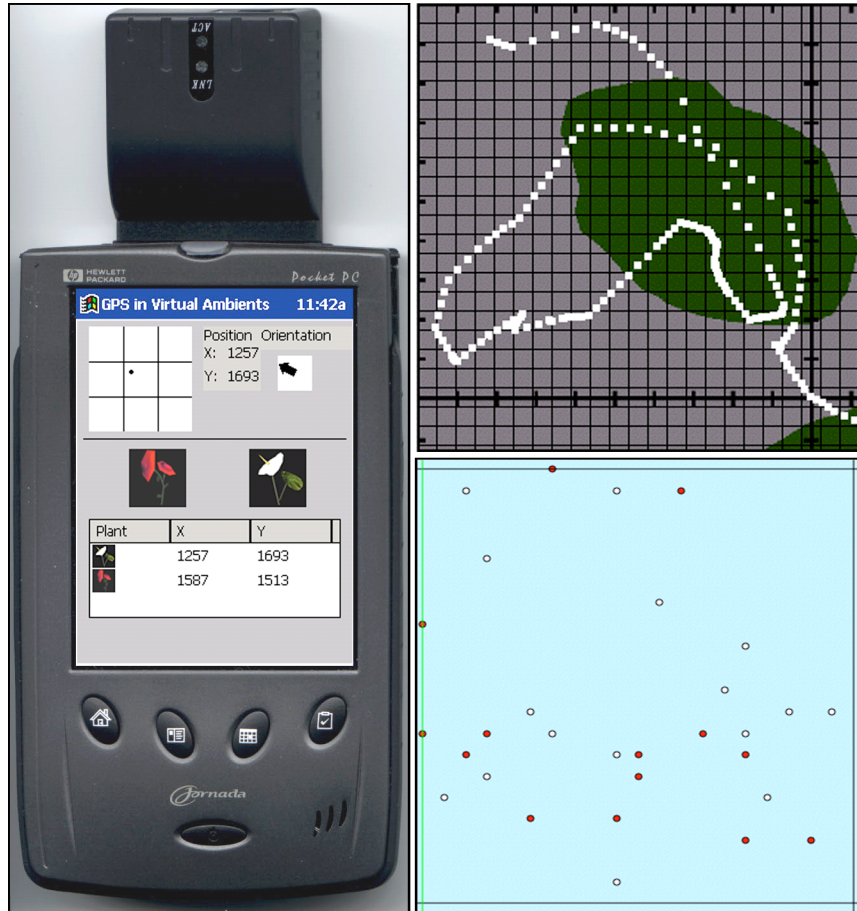
Figure 3: Aside from the ImmersaDesk, the students view three different displays during their survey. The Pocket PC acts as a GPS system showing the students' location and orientation in the Field as well as giving them the ability to record the plants that they find. The laptop map interface allows them to see where they have been. The laptop MyWorld interface allows them to see what plants they have found, and lets them see the interface they will use later to analyze the data.
