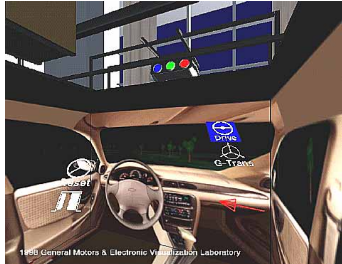
Figure 3. General Motors- VisualEyes. Shown is the inside of a virtual CAVE. By selecting this CAVE the participant will be teleported into the environment where the interior of a GM car is being designed.
