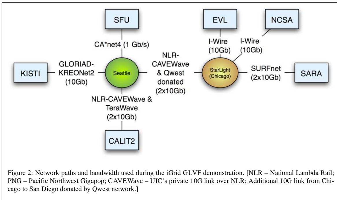
Figure 2: Network paths and bandwidth used during the iGrid GLVF demonstration. [NLR – National Lambda Rail; PNG – Pacific Northwest Gigapop; CAVEWave – UIC's private 10G link over NLR; Additional 10G link from Chicago to San Diego donated by Qwest network.]
