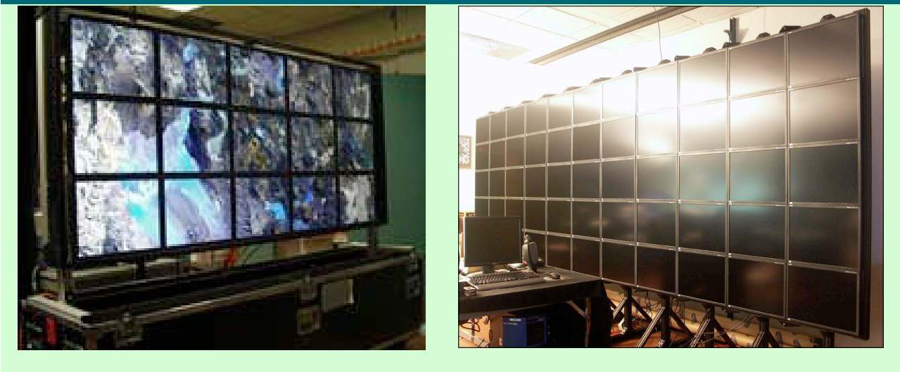
Figure 5 - Target high-resolution displays: GeoWall2 30Mpixels and LambdaVision 100Mpixels
