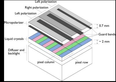
view of the main components of a micropolarized LCD 3D display
