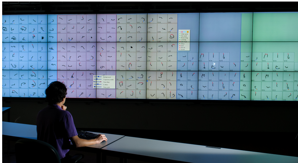
Fig. 1. Analysis of insect motion patterns on a 3D ultra-resolution display wall with a resolution of 19 Megapixels. Trajectories are juxtaposed in a small-multiples layout and grouped into bins depending on their associated meta data. The bins are given distinct background tint to distinguish them easily. The use of independent bins allows the user to explore multiple hypotheses in parallel.
