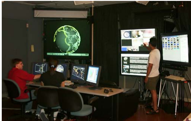
Figure 2: The Continuum- an Amplified Collaboration Environment. Top left is a passive stereo display for showing immersive 3D content; next to it are vertically stacked plasma screens that are used for AccessGrid video conferencing; to the right of this is the plasma touchscreen. The small screens in front of the students form a tiled display that can be mounted in a 2 X 2 matrix as show in Figure 6.
