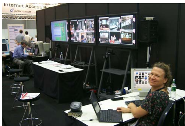
Figure 4: AccessGrid using plasma screens rather than projectors. This picture
