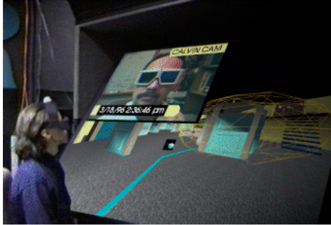
Figure 2: Participants communicate with audio and video over an ATM network using the ImmersaDesk
