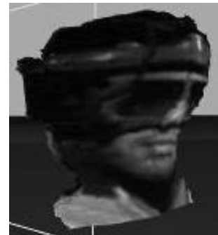
Figure 4. The OpenGL implementation of projective textures does not perform any visibility checks and hence the video is also mapped onto the occluded polygons. This causes the head to look distorted and thus it is necessary to avoid this.
