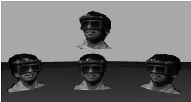
(b) The registration can be corrected by using the interactive tool. The tool lets the user adjust the registration in the X, Y and Z axis with its effect seen in real-time. Thereby, the registration can be corrected with ease. This process needs to be done only once after calibrating the camera.
