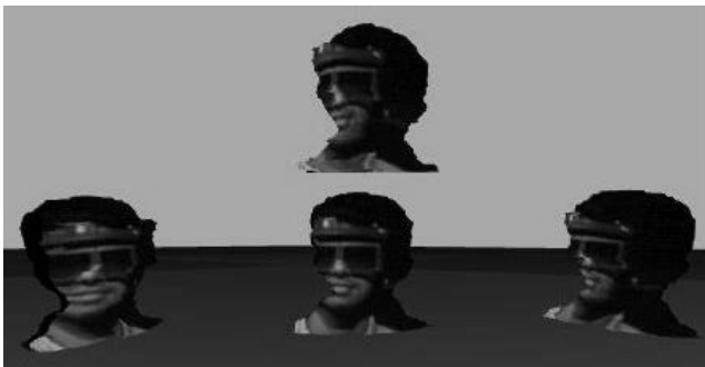
(a) Initial registration, using the camera parameters obtained by calibrating the camera, is not very accurate.
