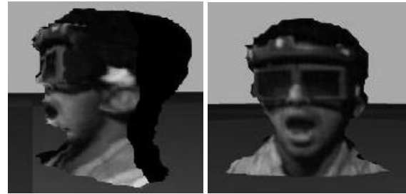
Figure 8. The image on the left shows the side view of the avatar where the error in registration is very noticeable when the jaw of the user is open. This occurs because the head model of the user is static. The image on the right shows that the error is not very noticeable from the front view of the avatar.
