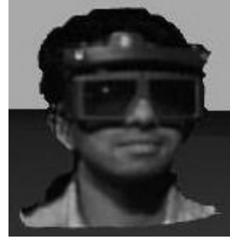
Figure 3. Projecting real-time video of the user onto the head model of the user to obtain a realistic avatar head.
