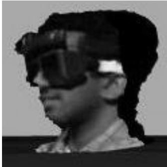
Figure 5. Projection of video onto occluded polygons is avoided by rendering the head in two passes. In the first pass, the occluded polygons are clipped and the frontfacing polygons are drawn with the projective textures enabled. In the second pass, the frontfacing polygons are clipped and the occluded polygons are drawn with a default texture.
