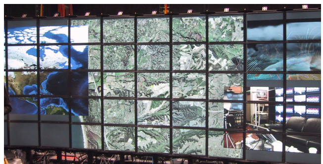
Figure 1. SAGE running on a 55-tile display in San Diego with applications streamed from Amsterdam and Chicago (iGrid 2005).
