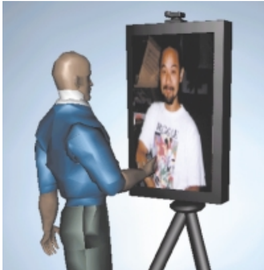
Figure 4. The AccessBot teleconferencing device. The remotely controllable pan-tilt-zoom camera mounted above the plasma display lets users look around the meeting room. AccessBot gives the remote user an equal presence with local meeting participants. —Image courtesy of Jason Leigh of the Electronic Visualization Laboratory
