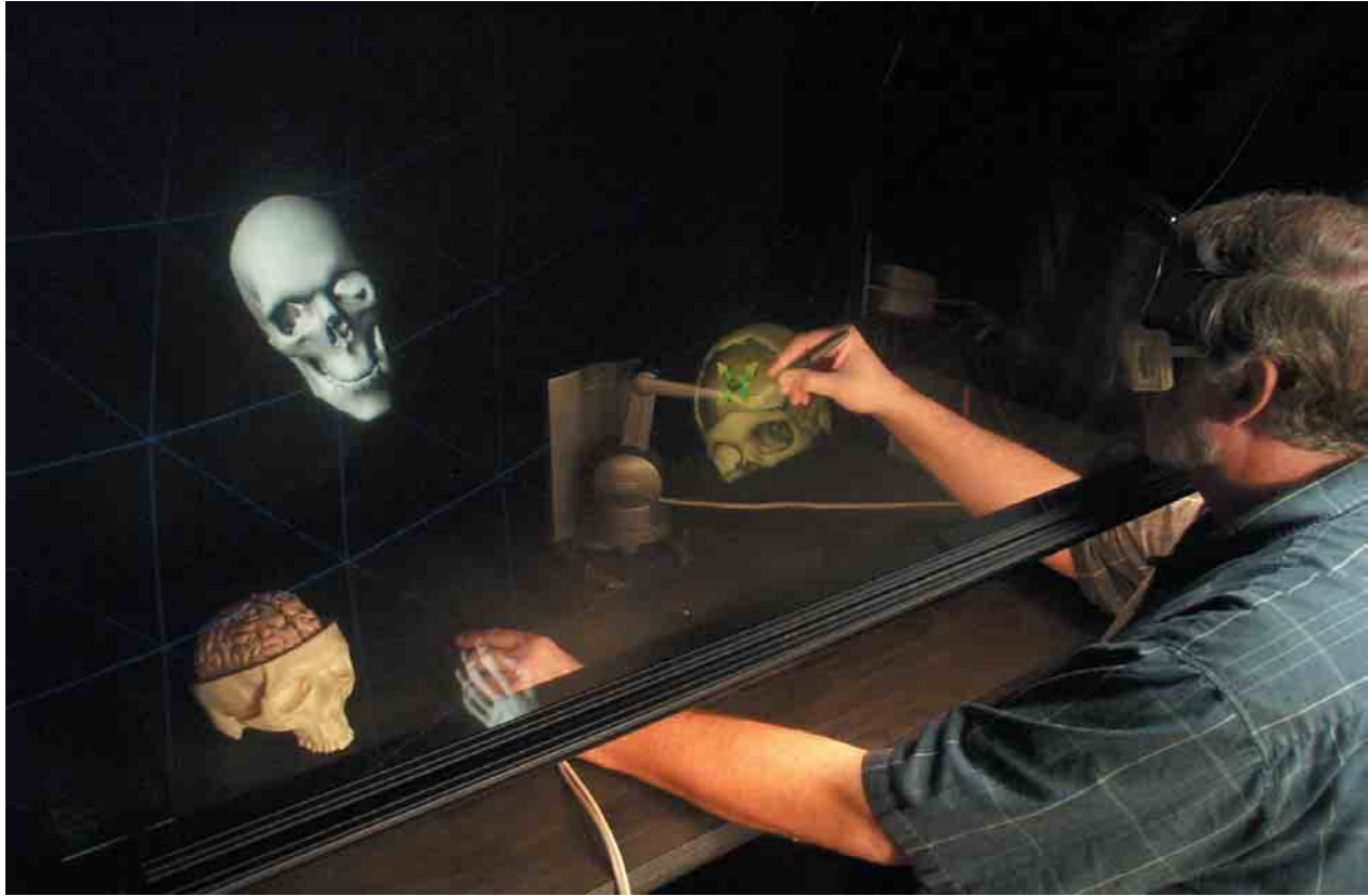
Figure 2. A medical sculptor “touches” a cranial defect while sitting at PARIS. The stylus corresponds to a tool held in the right hand, while a virtual hand tracks the position of the left hand. A real skull model remains visible on the table.
