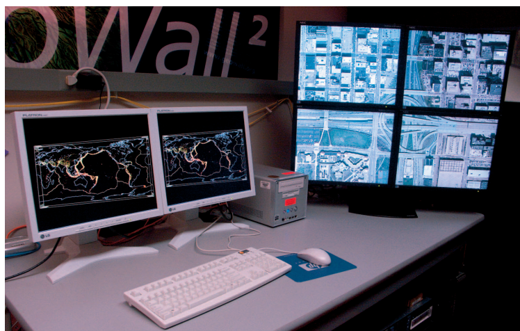
6 The Personal GeoWall-2 uses a single PC to drive both a classic GeoWall and a small 2 \times 2 tile display, giving the user a way to see both stereoscopic and high-resolution content simultaneously.
