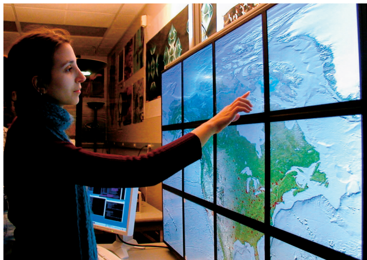
5 The GeoWall-2 addresses the need for high-resolution interactive imagery using an array of LCD panels driven by a cluster of PCs.
