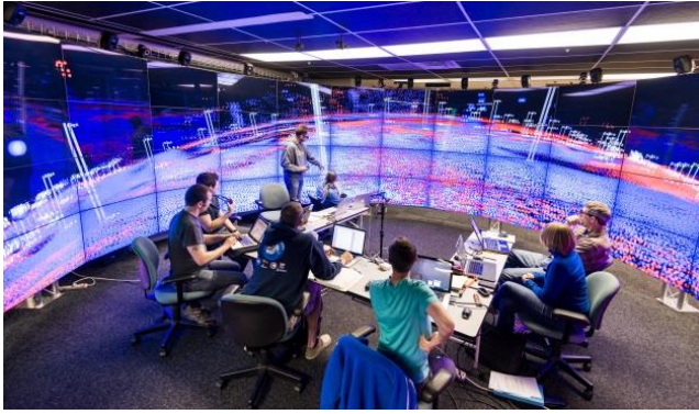
Fig. 5. Two photographs taken during a co-located collaborative meeting in CAVE2. On the left, an Omegalib immersive visualization is running on the full display. On the right, CAVE2 is split into two workspaces to display additional 2D views. Switching between the two modes can be done at runtime, without resetting running applications.
