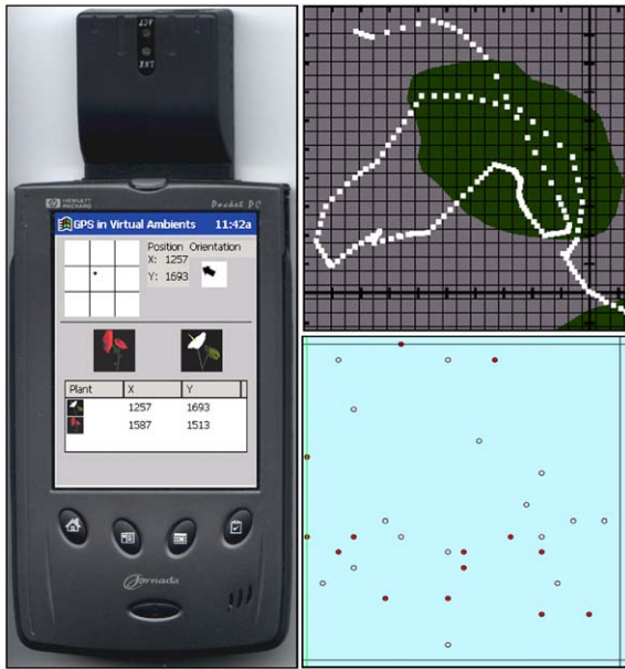
Fig. 3. Aside from the ImmersaDesk, the students view three different displays during their survey. The Pocket PC acts as a GPS system showing the students' location and orientation in the Field as well as giving them the ability to record the plants that they find. The laptop map interface allows them to see where they have been. The laptop MyWorld interface allows them to see what plants they have found, and lets them see the interface they will use later to analyze the data.
