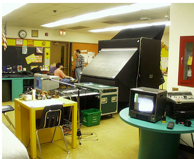
Figure 1: The ImmersaDesk and stereo monitor setup in the classroom
