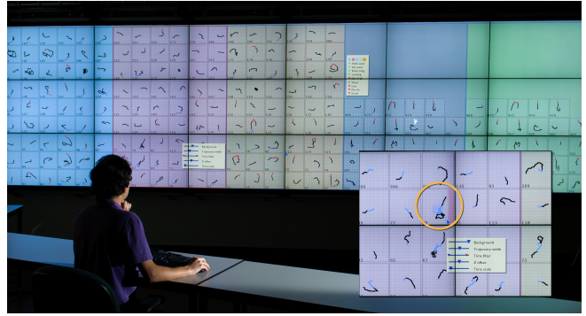
Figure 3. Our trajectory analysis application running on a 19 Megapixels, thin-bezel, tiled 3D display wall. Trajectories are juxtaposed side-by-side and grouped into “bins” depending on their associated meta data. A stereoscopic 3D visual encoding is used to convey spatial and temporal features in the trajectories. The frame at the right bottom of the figure illustrates Coordinated Brushing . A blue paintbrush (circled) is being used to highlight insect movement in the center of the experimental arena.
