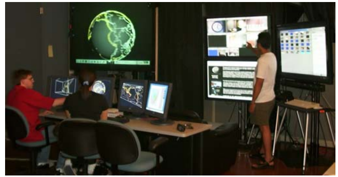
Figure 7: The Continuum. Top left is a passive stereo display for showing immersive 3D content; next to it are vertically stacked plasma screens that are used for AccessGrid video conferencing; to the right of this is the plasma touchscreen. The small screens in front of the collaborators form a tiled display that can also be mounted in a 2 X 2 matrix.
