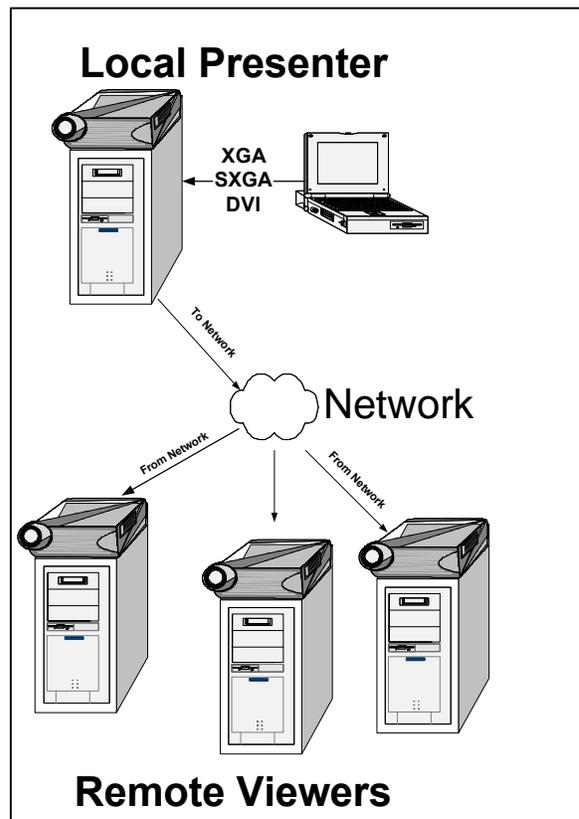
For the purposes of testing, the receiving end of the VBox is a Linux PC since our streaming software was originally developed for the Linux platform.
