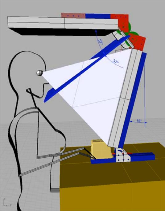
Figure 4: An Early Prototype Design of the ImmersaDesk-4. This version was actually built but was found to be structurally unstable.
