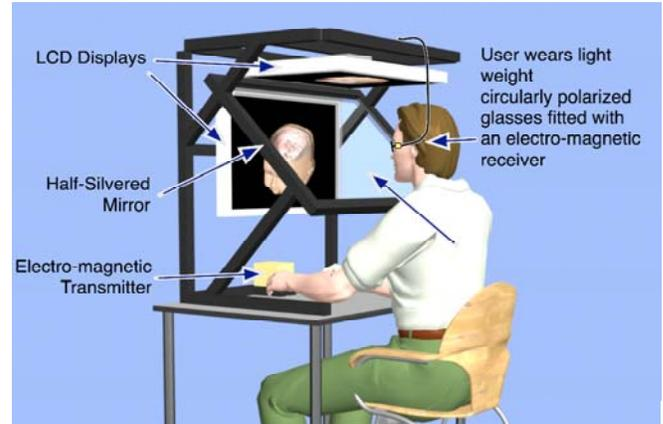
Figure 3: Schematic of the ImmersaDesk-4.
