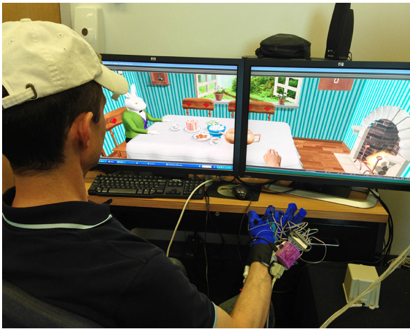
FIGURE 1. VR system and interaction with the immersive VR environment. Magnetic trackers are affixed to the baseball cap to track the head and to the PneuGlove to track the arm. Bend sensors on the PneuGlove provide digit joint angles. The scene is continuously updated according to these sensor readings.
