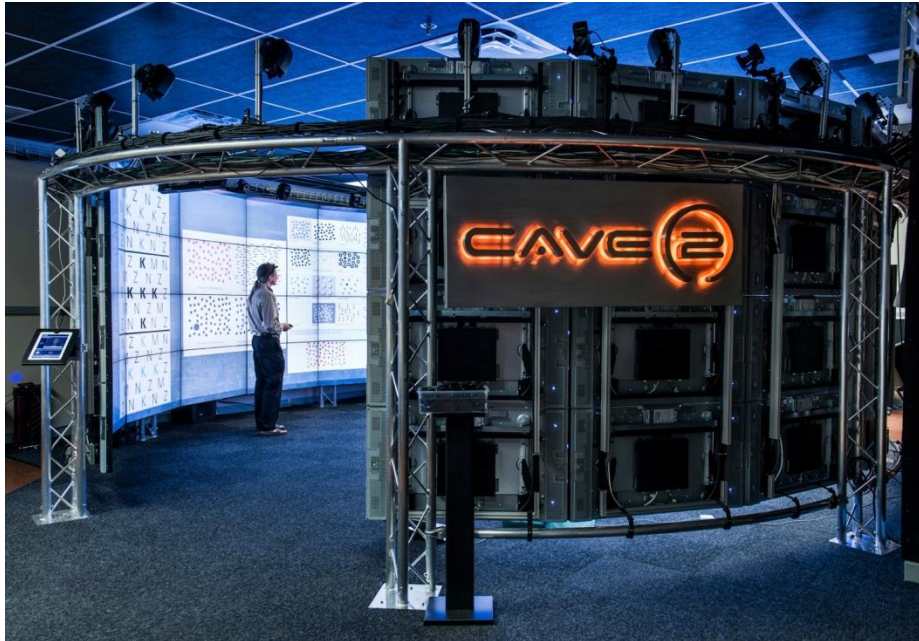
Figure 4. A picture of the implemented CAVE2 Hybrid Reality Environment
