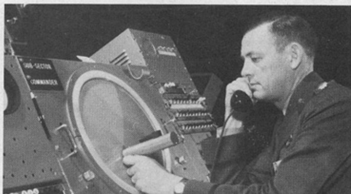
Figure 2. Experimental Sage operator consoles. This may be the first use of the light pen in computer graphics. (Photo courtesy of Mitre Corp.)
