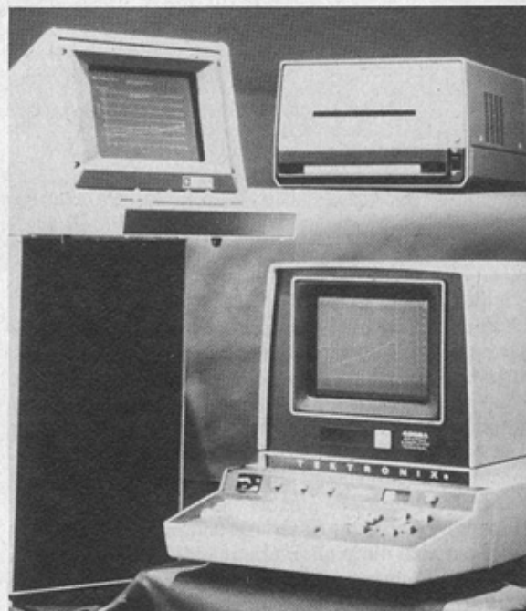
Figure 11. Early Tektronix computer graphics products. T4002A, lower righthand corner; T4010, upper lefthand corner; 4610 hardcopy unit, upper righthand corner. (Photo courtesy Tektronix)
