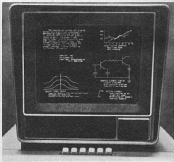
Figure 10. Comptek, Inc., Model 400 storage tube terminal. (Photo courtesy of Comptek)
