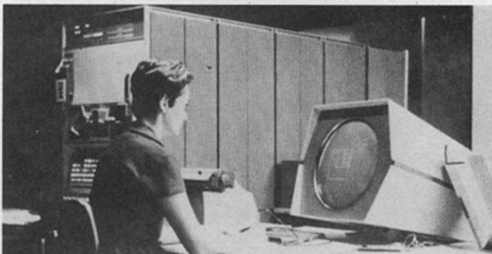
Figure 3. Digital Equipment Corporation Type 30 display (early 1960's). (Photo courtesy of Digital Equipment Corp.)
