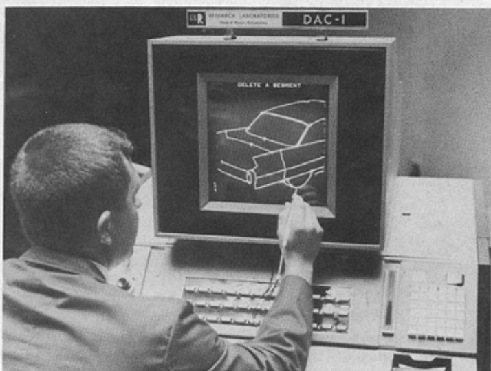
Figure 4. General Motors DAC/1—Design Augmented by Computer—installation. (Photo courtesy of GM Research Laboratories)
