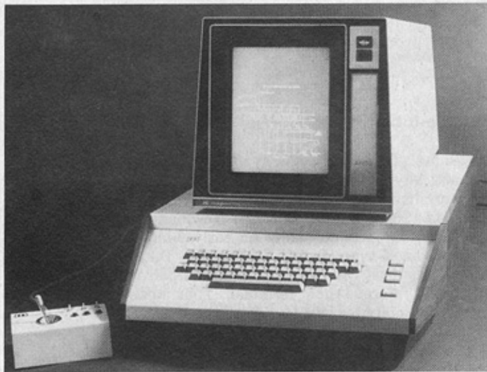
Figure 9. ARDS terminal manufactured by Computer Displays, Inc. First "low cost" storage-tube-based graphics terminal. (Photo courtesy of Adage, Inc.)
