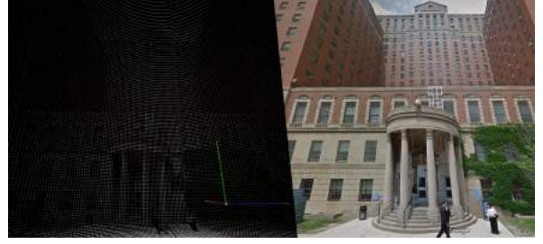
Figure 4. Comparison between a sample building reconstructed as a point cloud and the original displayed on Google Street View
