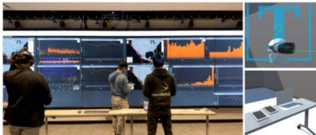
Figure 15: Subjects examining a set of created visualizations while using different devices. Position and orientation of subjects and devices are streamed from OptiTrack Mocap system to a Unity application depicting a 3D model of the physical space.
