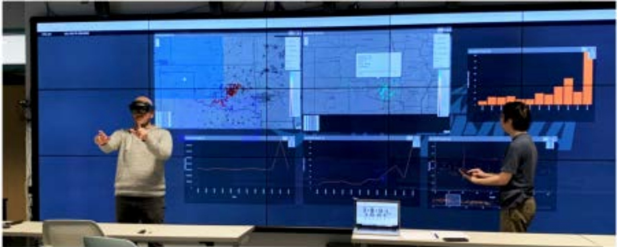
Figure 13: In a collaborative session, the user on the left is examining data in 3D using a HoloLens device. Data points (Wells) within the blue rectangle on the left map are viewed in 3D via HoloLens. The other user on the right is using a tablet (with linked visualization) to inspect specific areas on the right map.
