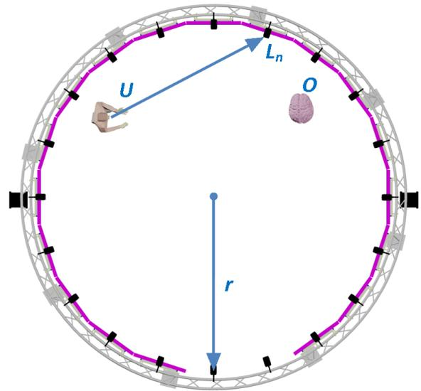
Figure 3 The distance between the user and loudspeaker is divided by the radius of the CAVE2. This ratio is squared to find that loudspeaker's amplitude weighting.
