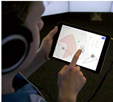
Figure 2. A user exploring the augmented reality in a CAVE system, while using a mobile device to edit the 3D sonic virtual reality he is hearing through headphones. The user is controlling the position of an object in lateral-view mode.
