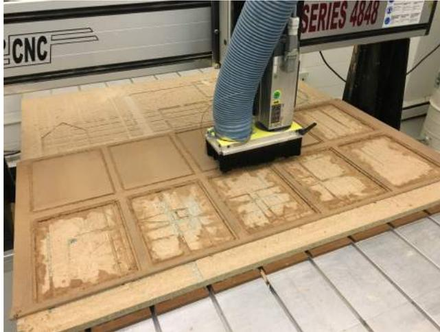
**Figure 3:** The MDF framework of the sculpture being milled with a CNC machine.
