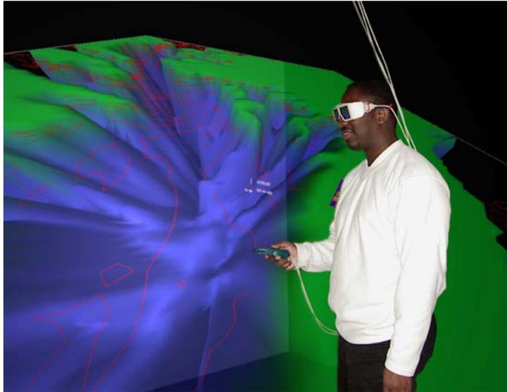
Figure 2. EVL's projection-based, first-in-kind CAVE VR system was used in conjunction with the Visualization Toolkit (VTK) to interactively analyze geospatial data collected from the Chesapeake Bay. Note the wired glasses and controller, and the low-resolution of the environment. The CAVE size was 10 ft (or 3m) cubed.
