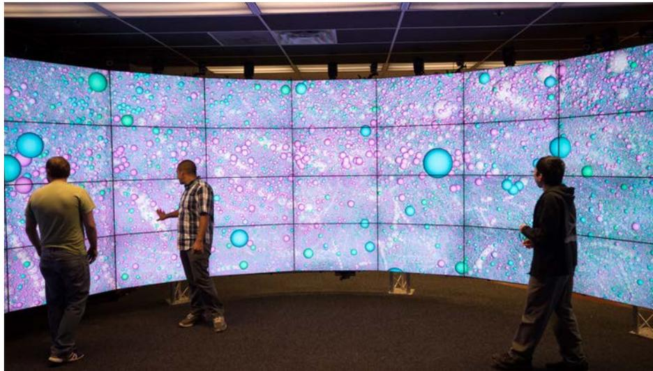
Figure 4. CAVE2 immersive exploration of dark matter formation in the universe. Note that while little information can be shown on a typical desktop display (one rectangle in the 320-deg. wall shown), the high-resolution tiled environment allows analysts to examine detailed information without losing the context of the larger dataset. Analysts (team of 7, not all shown here) also appeared to use kinesthesia to navigate through this space.
