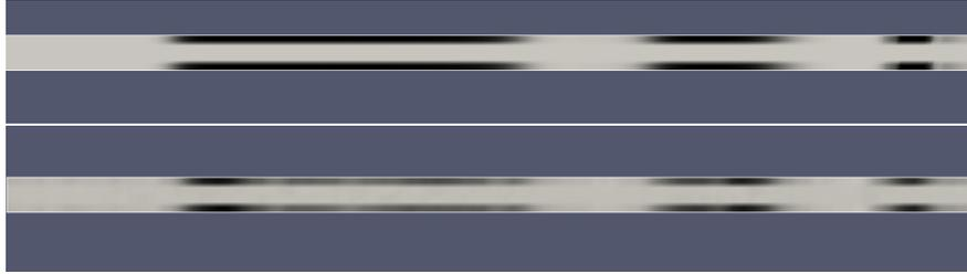
**Fig. 7** The network comparison between the network ground truth (top) and the final reconstruction (bottom) for the 100th time-step of the 3D SOD dataset. The dark narrow bands seen in the two images indicate large density gradients, and correspond to potential shock regions. Note the three distinct shock zones in the images.
