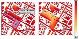
Fig. 11. Comparison of the impact of nearby buildings on the overshadowing of Yvette Chauviré Square Park (left) with an alternate scenario of without the buildings (right). The buildings considered are highlighted in purple. Removing these buildings too close to the park improves sunlight access by a significant amount.
