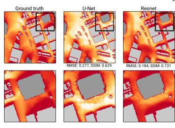
Fig. 5. Results of ablation study using U-Net and ResNet generator architecture and  $L_1$  loss function. RMSE and SSIM scores with respect to ground truth are highlighted below each image (for SSIM, higher values are better). Note that ResNet architecture produces significantly better results, especially for longer shadows that are distant from the building. Top: Highlights with areas with longer shadows. Bottom: Zoomed areas.
