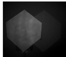
Figure 6. Photographic measurement of crosstalk. Primary channel is a brighter cube at the left and the crosstalk to its right shows a faint ghost image.
