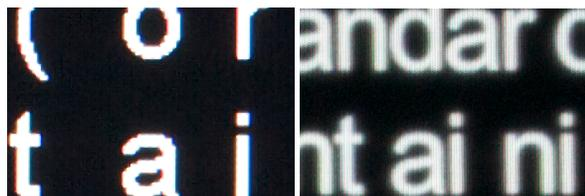
Figure 7. Comparison of text displayed in 2D on a comparable single-layer LCD monitor (left) and similar text displayed in 2D on our Dynallax system (right) reveals significant light dispersion due to internal reflections.
