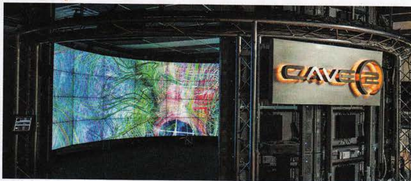
The brain's neural fiber tracts are shown on 72 3-D LCD screens that line the inside of a 24-foot-wide, 8-foot-tall, 320-degree room at the University of Illinois at Chicago.
