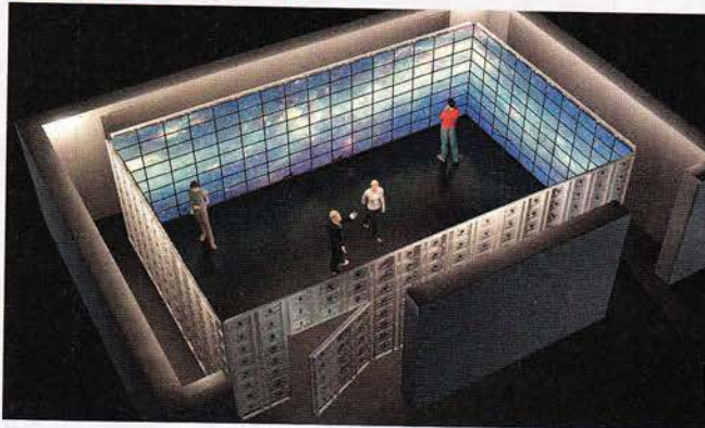
The Reality Deck's 627 square feet are tiled floor-to-ceiling with 416 high-resolution monitors. Its total resolution is more than 1.5 billion pixels.
