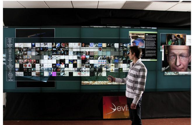
Fig. 9. The media browser, developed using SAGE widgets, is a tool for easily browsing and showing multimedia files on large high-resolution displays.
