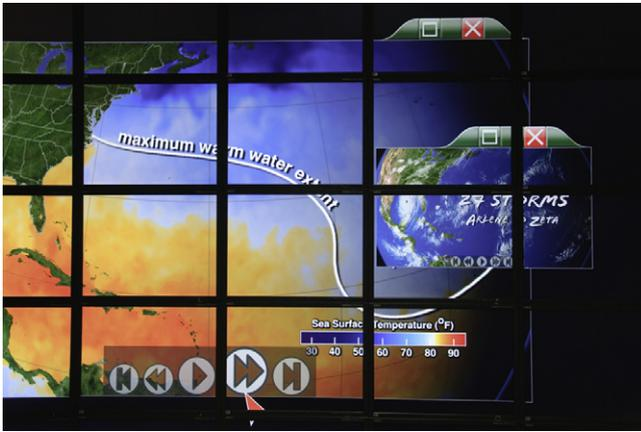
**Fig. 6.** Application widgets are scaled relative to the application window (player controls) while global widgets are scaled relative to the display size (maximize and close buttons).
