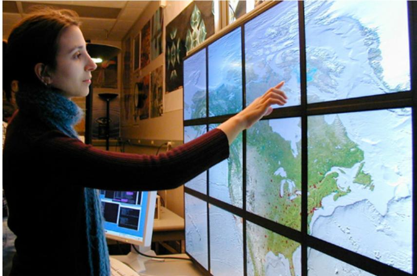
Figure 5: The GeoWall-2 addresses the need for high-resolution interactive imagery utilizing an array of LCD panels driven by a cluster of PCs.
