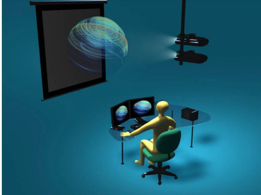
Figure 3: The GeoWall uses two DLP projectors connected to the dual outputs of a PC-based graphics card to generate stereoscopic visuals. Filters are attached to the projectors to polarize the light which is then projected onto a polarization-preserving screen. Viewers wear lightweight polarized glasses to correctly view the imagery in stereo.
