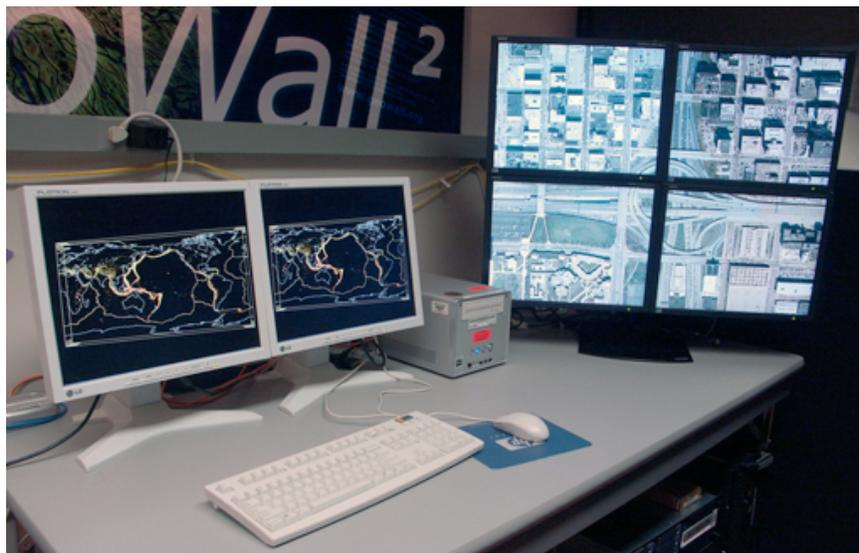
Figure 6: The Personal GeoWall-2 uses a single PC to drive both a 'classic' GeoWall and a small 2x2 tile display, giving the user a way to see both stereoscopic content and high-resolution content simultaneously on a single PC
