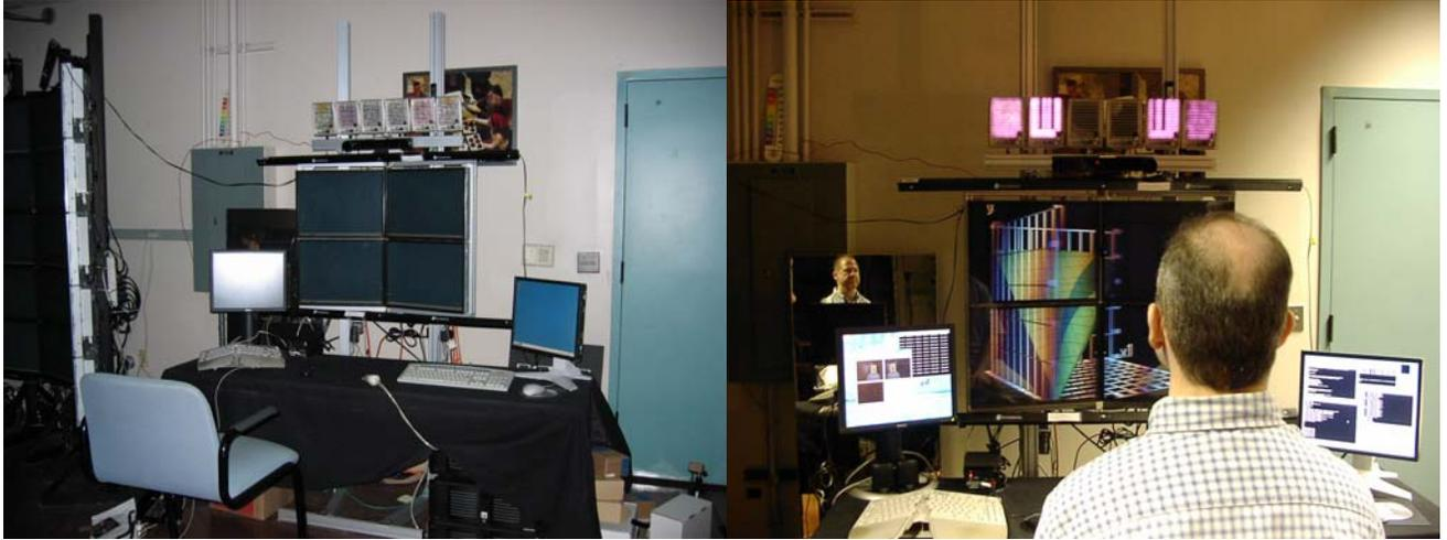
**Figure 1.2:** EVL's Varrier™ Autostereo Virtual Environment turned off (left) and turned on with a user (right).
