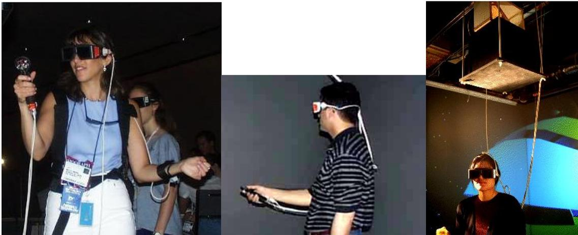
**Figure 2.1:** Hand-tracker system attached to a wand and a head-tracker system attached to a stereo-glasses.
