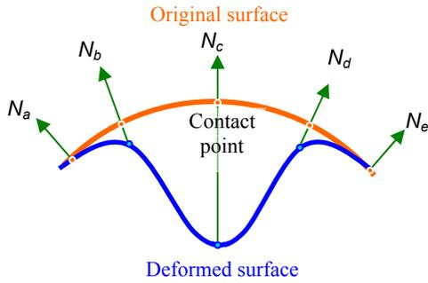
Fig. 2. Vertex displacements along its normals  $N_i$  done by the vertex shader
