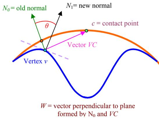
Fig. 5. Normal calculation done by the fragment shader
