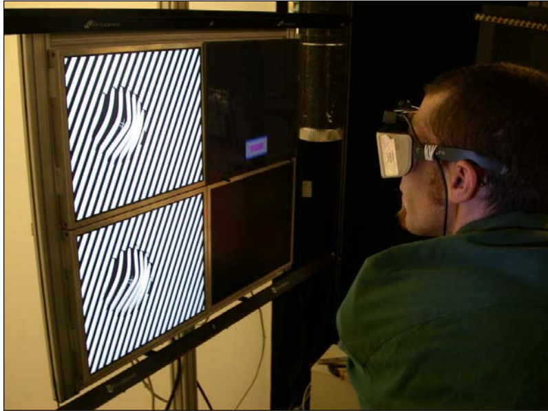
Figure 8: Varrier software is used with AGAVE (Access Grid Autostereo Virtual Environment), a panel-based, head-tracked, barrier-strip auto-stereographic display. The viewer does not wear stereo glasses (in the picture, the head-tracking hardware is attached to the glasses' frame, but the glasses have no lenses). The screen shows a magnified version of a virtual line screen.
