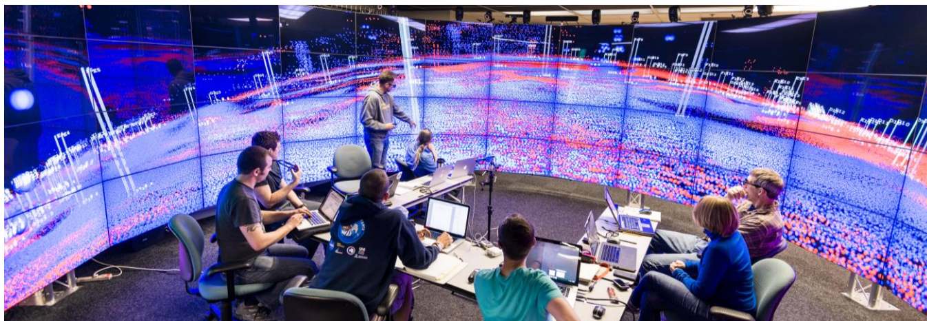
Figure 1. A team of environmental scientists analyzing sonar data from West Lake Bonney, Antarctica using our visualization tool inside the CAVE2 hybrid immersive environment. The full dataset consists of 350 million sonar points, which can be filtered interactively based on attributes such as ping return time, beam takeoff angle and timestamp. The point cloud is overlaid with a secondary depth data source (the white columns) for cross-checking sonar depth accuracy.
