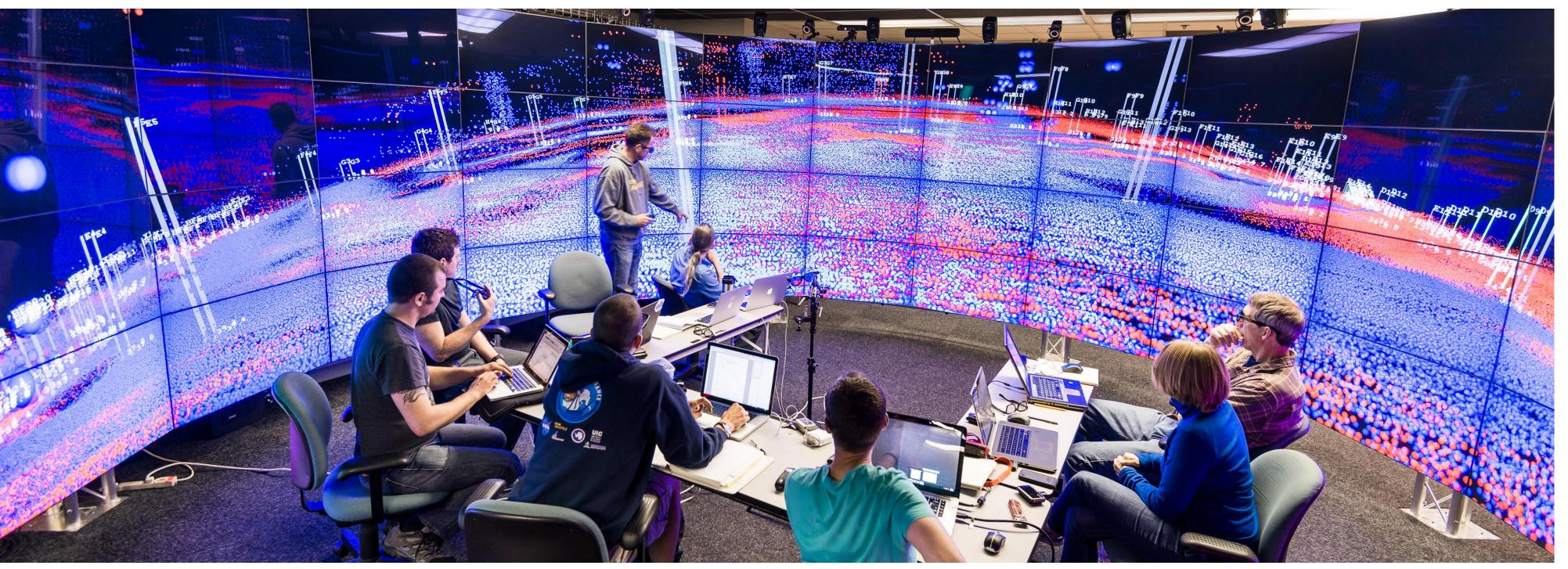
**A team of environmental scientists analyzing sonar data** from West Lake Bonney, Antarctica using our visualization tool inside the CAVE2 hybrid immersive environment. The full dataset consists of 350 million sonar points, which can be filtered interactively based on attributes such as ping return time, beam takeoff angle and timestamp. The point cloud is overlaid with a secondary
