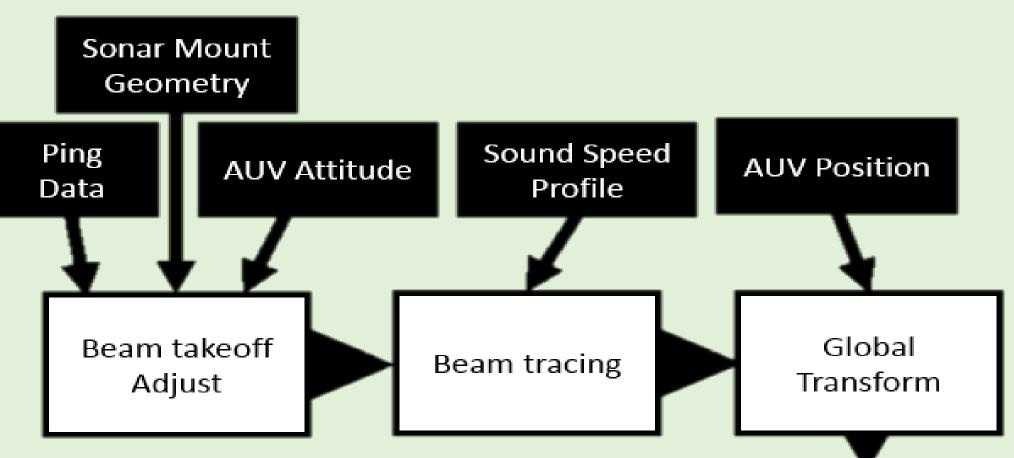
characteristics. After beam tracing, the 3D points generated from multiple missions are merged into a single point cloud: overlapping data is used to filter noise and to generate final output points at the desired resolution level.
