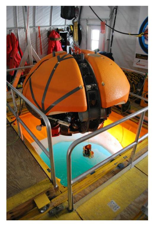
Environmentally Non The **Disturbing Underwater Robotic ANTarctic Explorer (ENDURANCE)** AUV was deployed in West Lake Bonney, a perennially ice covered lake in Antarctica and operated on science objectives: water chemistry profiling, bathymetry scanning, and glacier exploration. For the purpose of bathymetry reconstruction, the source data consisted of about 350 Million distinct sonar range returns, plus navigation data and AUV attitude information at 0.2 second intervals.
