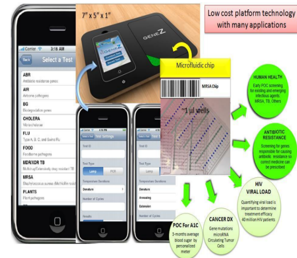
Figure 1: Gene-Z™: Hand-held genetic diagnostics (LAMP or PCR), iPod user interface, disposable chips.
