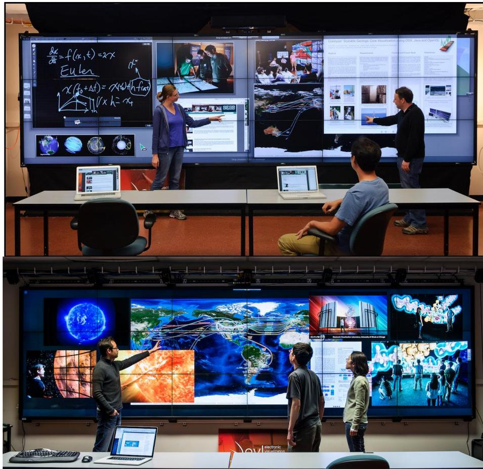
Figure 3. A single machine-driven tiled-display wall run by SAGE (top) and SAGE-Next (bottom) at the Electronic Visualization Laboratory in the University of Illinois at Chicago. The 20' by 6' display wall is made up of 18 LCD panels with a total resolution approximately 18.8 megapixels.
