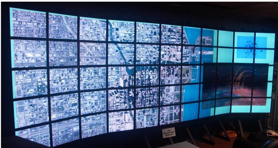
Figure 1. The 100-megapixel LambdaVision tiled-display wall driven by a cluster of 28 computers and run by Scalable Adaptive Graphics Environment (SAGE).
