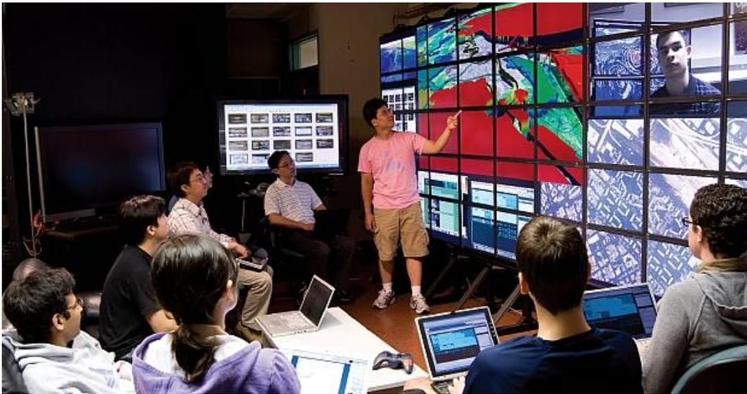
Figure 5. 100-megapixel LambdaVision display used in a research meeting at the Electronic Visualization Laboratory at the University of Illinois at Chicago. The participants stream their desktop screens to the display wall using VNC. Multiple visualizations and HD video of remote participant are streamed to the display wall.
