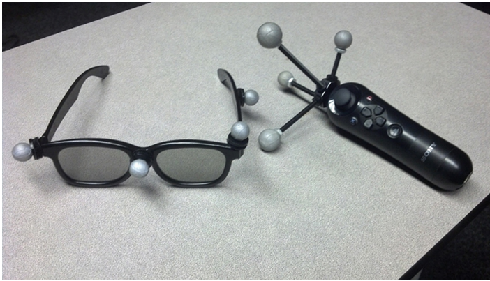
Fig. 2. CAVE2 input devices; the head and the wand controllers with retro-reflective markers for Vicon infrared optical tracking system.
