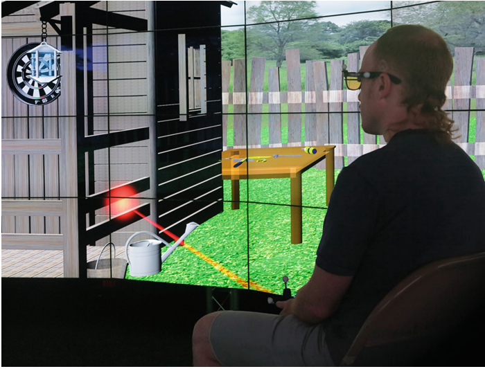
Fig. 5. Direct manipulation interaction in the CAVE2. By pushing a button on the Wand, the performer can point the virtual laser pointer and click on the watering can trigger object.
