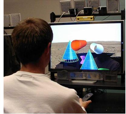
**Figure 5: A user is seated at the Personal Varrier system, designed in a desktop form factor to be used comfortably for extended periods of time. Autostereo together with camera-based tracking permits the user see 3d stereo while being completely untethered.**
