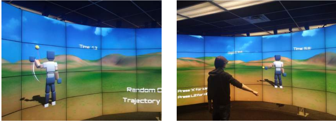
Figure 4: Left: When Trajectory Mode is enabled, the movements of the avatar generate white trails disappearing after a certain amount of time. At the same time, a red ray highlights the optimal trajectory to reach the current target. Right: In this example, the Distorted Mode maps the movement of the right part of the body of the patient to the left part of the avatar.
