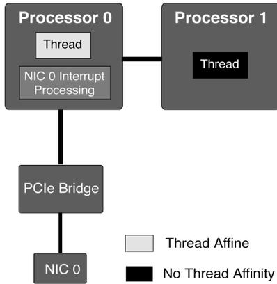
Figure 4. This figure depicts the Thread Affinity (TA) property. TA is set if the network application thread is bound to the processor where the interrupt processing occurs
