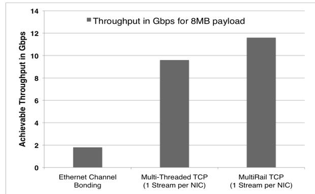
Figure 11. Performance evaluation of 2 x 10GE Linux Ethernet Channel Bonding, user-space Multi-Threaded TCP over 2 NICs and user-space MultiRail Library based TCP over two network rails for transferring a payload of 8MB.
