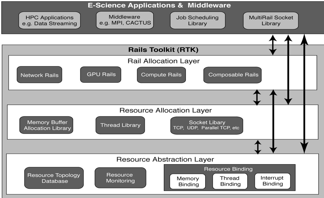
Figure 2. Rail Toolkit Architecture. This figure depicts the various layer in the design of the Rail Toolkit (RTK) architecture. RTK consists of Resource Abstraction Layer, Resource Allocation Layer and Rail Allocation Layer. E-Science applications and middleware can use any of the 3 layers for optimizing their performance to an end-systems topology.
