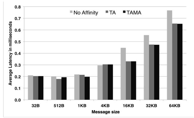
Figure 7. Effect of affinities on the latency of multiple UDP streams. Thread affinity plays a key role in improved throughput
