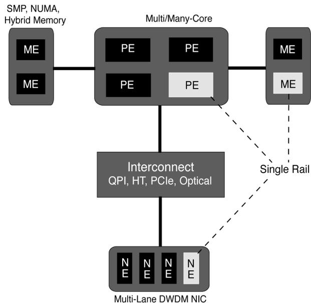
Figure 1. The Rails approach. This figure depicts a network rail wherein co-allocation of memory elements (ME), processor elements (PE) and networks resources (NE) help achieve improved performance
