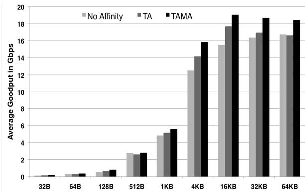
Figure 9. Effect of affinities on the aggregate goodput (throughput with 0% packet loss) of four concurrent UDP streams. As payload increases, enabling affinities leads to a higher performance in comparison to a default Linux system.
