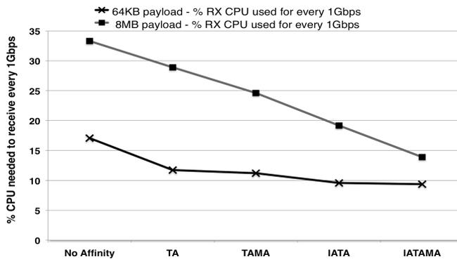
Figure 10. Effect of affinities on the average CPU Utilization of four concurrent TCP Streams to process 1Gbps. Using RTK, the application needs less CPU to process 1Gbps TCP traffic.
