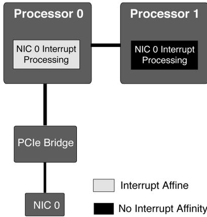
Figure 3. This figure depicts the Interrupt Affinity (IA) property. IA is set if the interrupt processing occurs on a processor where the device is physically connected
