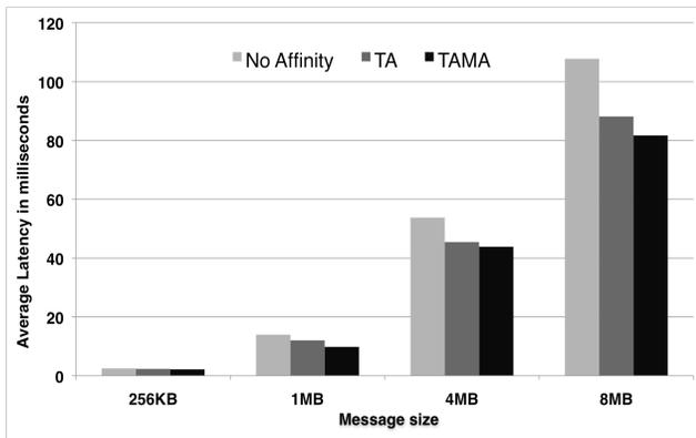
Figure 6. Effect of affinities on the latency of multiple TCP streams. As the message size increases, memory affinity is key for improved throughput
