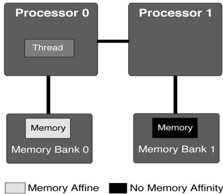
Figure 5. This figure depicts the Memory Affinity (MA) property. MA is set if the application buffer is allocated on the memory bank where the network application thread is bound.
