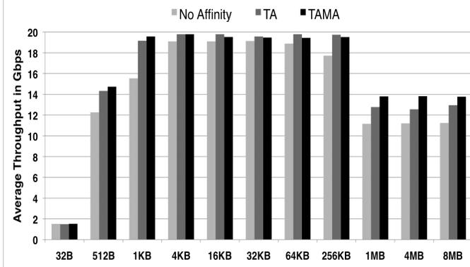
Figure 8. Effect of affinities on the aggregate throughput of four TCP streams. As the payload size increases, enabling affinities leads to higher throughput in comparison to a default Linux system.
