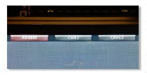
At the top of the SAGE interface are tabs which are used to connect to SAGE collaborators for sharing of SAGE content. SAGE sessions are shared by connecting to SAGE user IP addresses. These connections can be made to 'All sites' or to individual sites set as default collaborators via interface customization. Files are shared by dragging and dropping onto the tab of the desired location.
