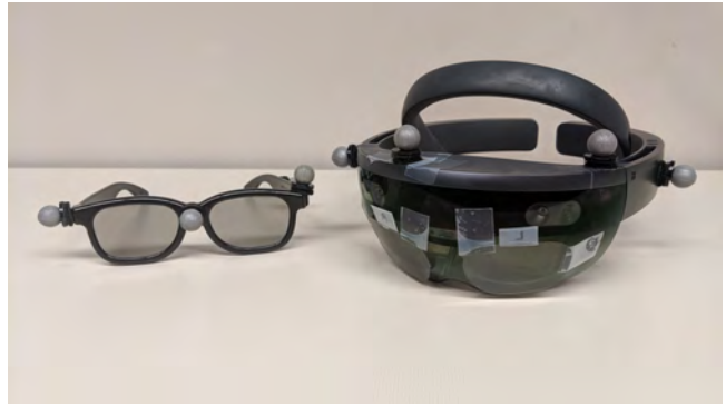
Figure 1: Standard CAVE2 glasses (L) and retrofitted HoloLens (R) with optical tracking markers and passive stereo lenses
