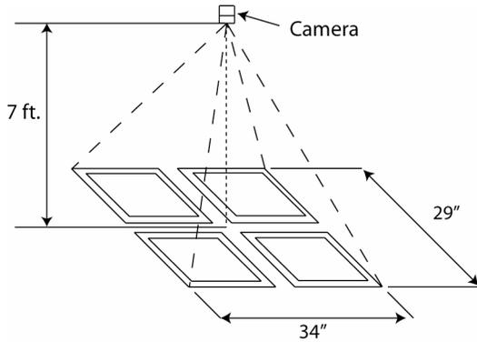
**Figure 3. The smaller table implementation for conducting a Fitts' test.**
