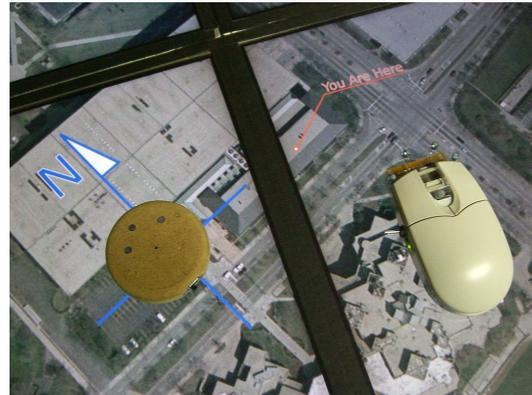
**Figure 2. Two tracked tangible devices; an orientable compass rose and a direct pointing device.**
