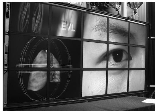
**Figure 5. Demonstration of three TeraVision servers streaming video to three different sections of the tiled-display. Each video stream is independent of each other but the screens for each stream are synchronized.**
