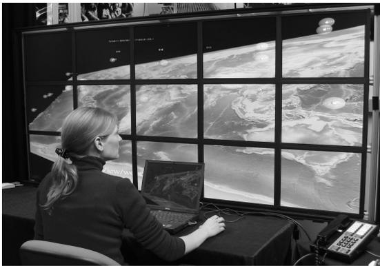
**Figure 4. A user streams her 1600x1200 laptop screen to Electronic Visualization Laboratory's 6400 x 3072 pixel tiled display at 10 fps.**
