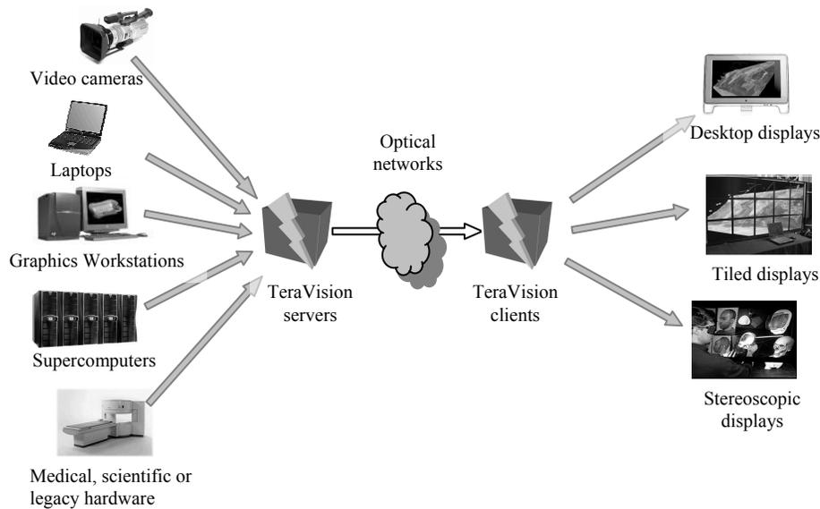
**Figure 1. TeraVision servers can stream video from a variety of video sources and automatically resize the video stream to fit the client displays.**
