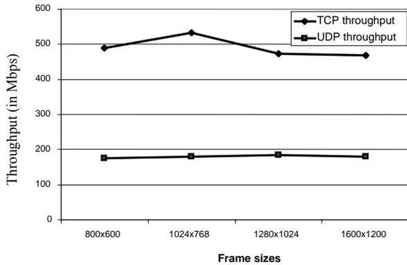
**Figure 8. TeraVision throughput for different frame sizes.**
