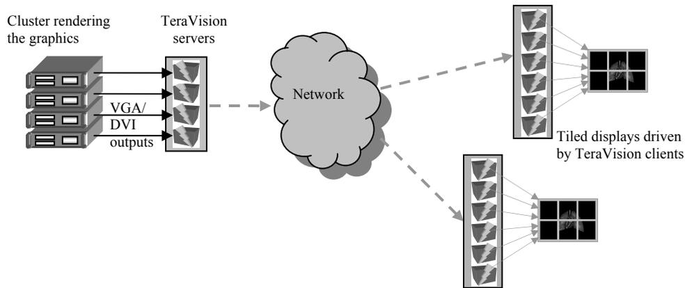
**Figure 3. Example of streaming tiled displays using multiple VBoxes at each site.**
