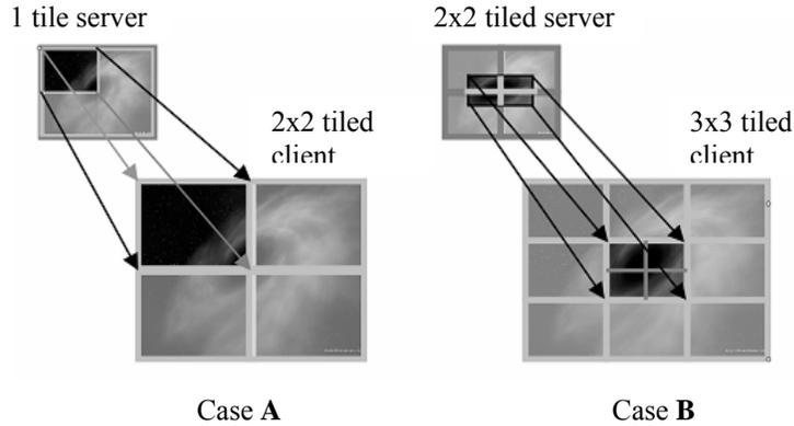
**Figure 7. Case A depicts a single tile server sending its video to a 2x2 client. In this case the server has to service 4 clients and each client connects to one server. In the second case, the server is a 2x2 tile configuration and the client is a 3x3 tiled display. If we consider the center tile on the client, we see that it has to receive 4 video streams from 4 different servers.**
