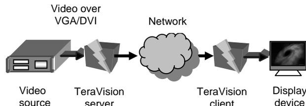
Figure 2. Typical TeraVision setup
